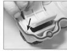
4.5 Ensure the gasket is correctly located in the camshaft cover recess (arrowed)
