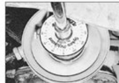
5.6 Fit the new retaining bolt and tighten it as described in the text
