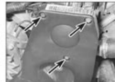
6.2 Timing belt upper cover retaining bolts (arrowed)
